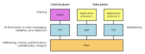
Protocol stacks for control and data planes if using IPsec.
