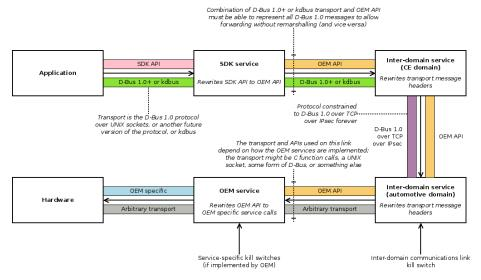
Apertis IDC message flow, following a message being sent from application to hardware; the message flow is the same in reverse for message replies from the hardware
